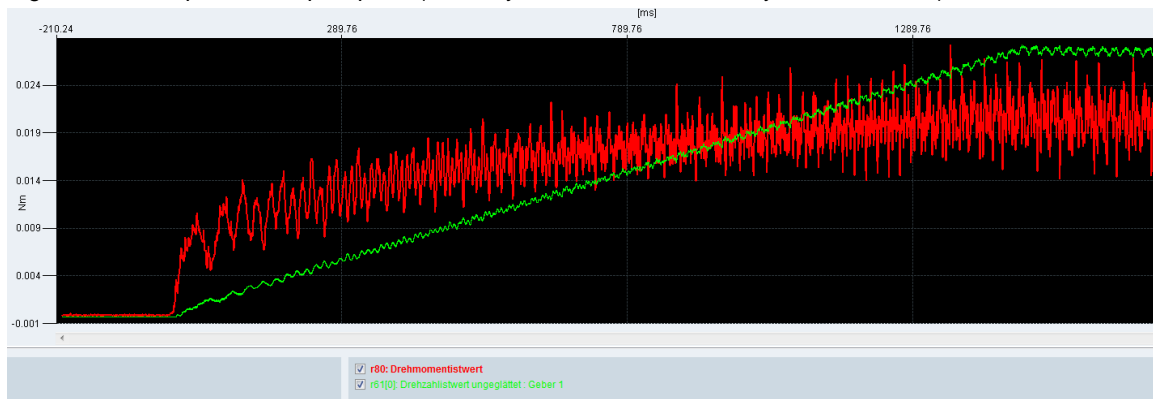
Figure 3-7 Example 2 of torque/speed (OB91 cycle time = 10 ms; bus cycle time = 4 ms)
